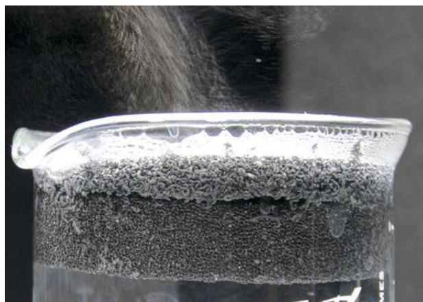
*Solar sponge: The top layer of graphite soaks up the sun's energy in tiny holes. When drops of liquid fill the holes, the water quickly evaporates. (The beaker looks hot, but the water below the sponge is cool).*
